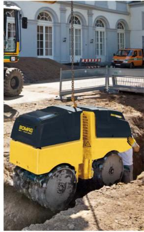
Safe and easy to transport with stable single-point lifting.
